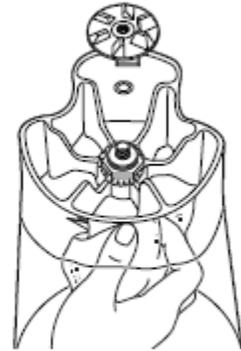
Remove the clutch and felt washer.
