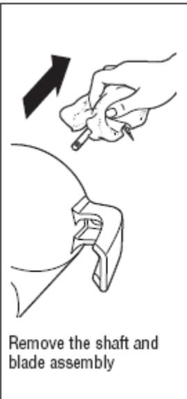
Remove the shaft and blade assembly
